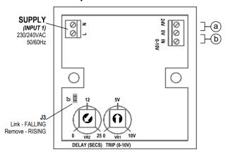
DELAY TIMER (0-25 Seconds) Delays operation of Alarm (to prevent nuisance switching). Set to zero (0) for instant ON.
