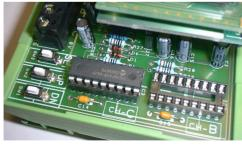
The example above shows CAD-XM1 expansion fitted to IC3 thereby enabling Channel-C.
