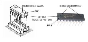
The CAD-XM1 expansion chip has to be installed orientated the correct way around. Whilst fitting the chip incorrectly will not do any damage, it will not do any good either since the Channel will not work until it is correctly installed.
