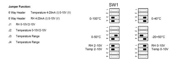
Note: for 4-20mA operation SW1 & 2 must be set to 2-10V
