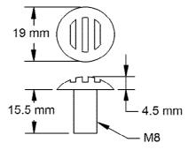
**Note:** the sensor is fully potted internally in the housing so if correctly sealed to a surface when mounted it is IP65
