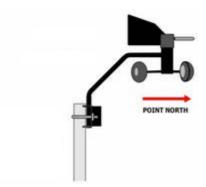
Mount the wind sensor, with its arm pointing North using the supplied compass.
