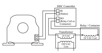
will not need to be externally powered, since the power for the switch is induced from the conductor being monitored. Another great feature of these current switches is that they include a Red "Status" LED that will indicate whether the current is above or below the fixed trip point. All of these units come with a unique 35 mm Din Rail mounting flange and an unconditional 5 year limited warranty.
