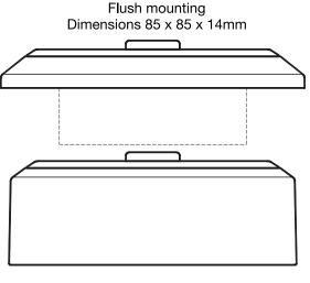
Surface mounting Dimensions 80 x 80 x 32mm
